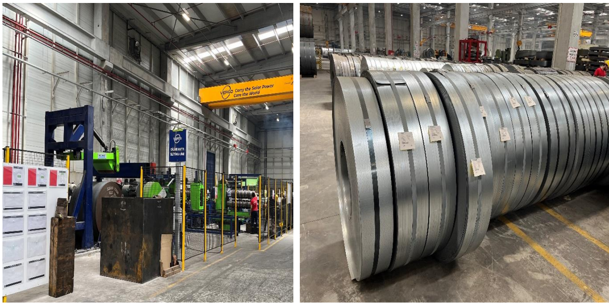
Figure 4. Slitting Line and Sliced Roll Sheet
