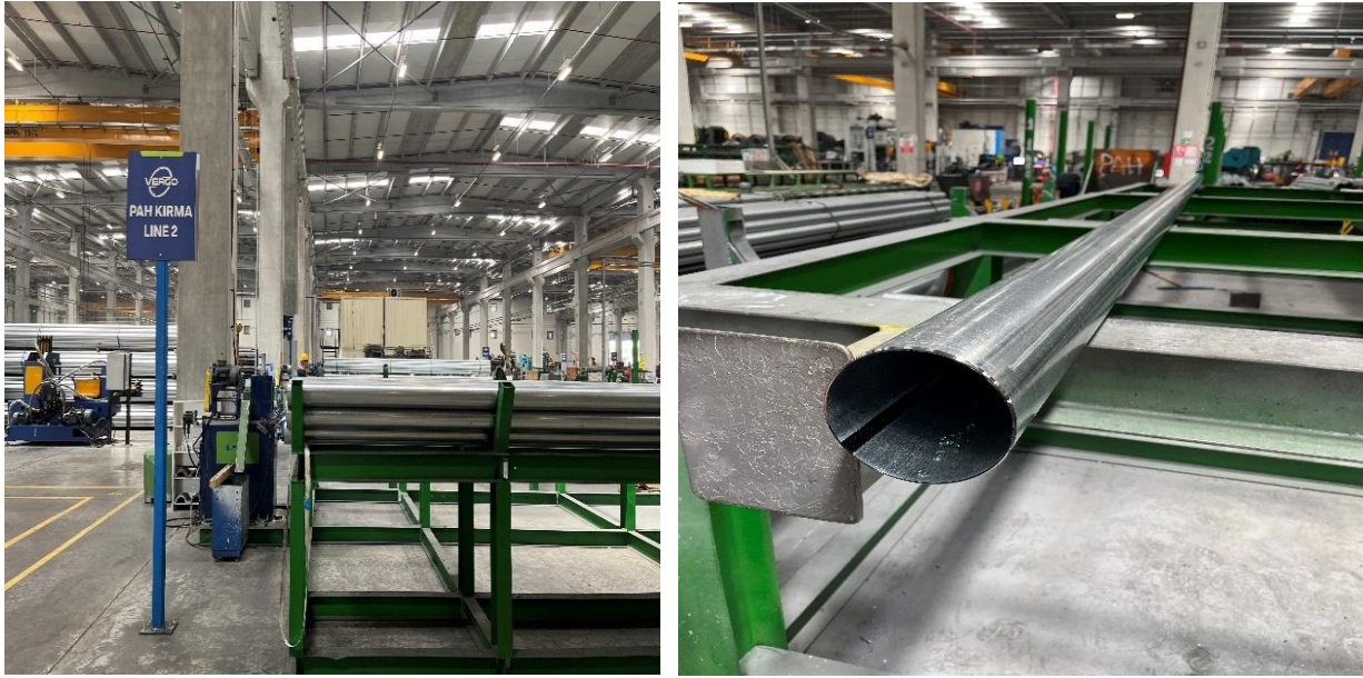
Figure 10. Chamfering Line for Pipes
