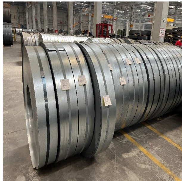
Figure 4. Slitting Line and Sliced Roll Sheet
