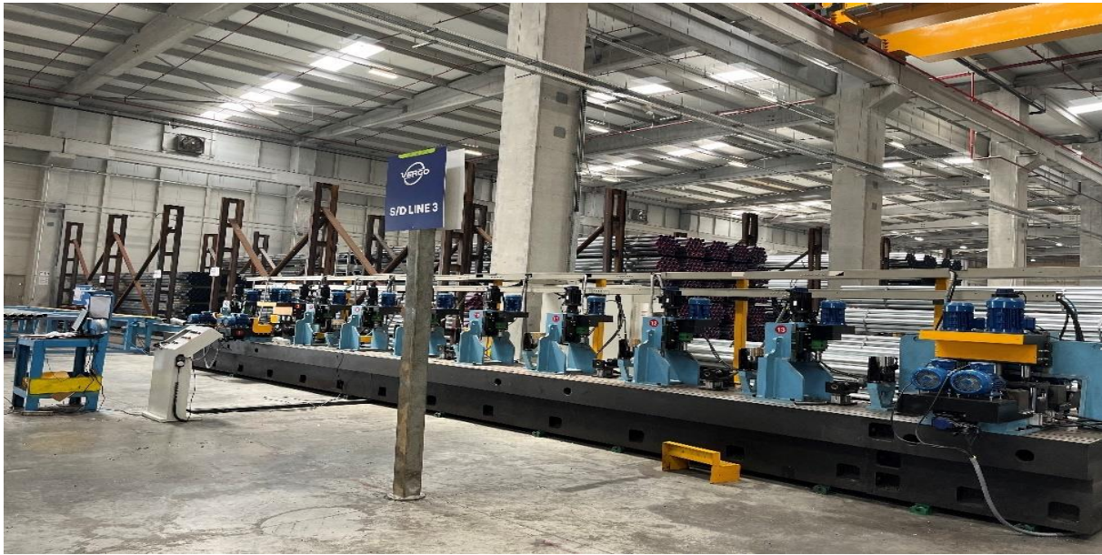
Figure 9. S&D Line for Spinning and Drilling of Pipes
